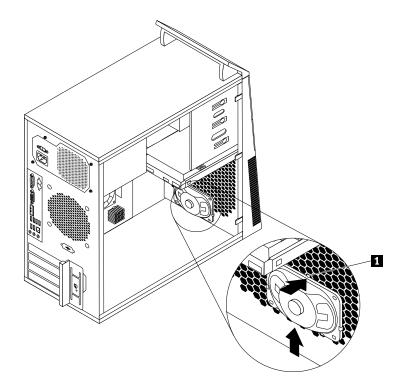
Figure 46. Removing the old internal speaker
